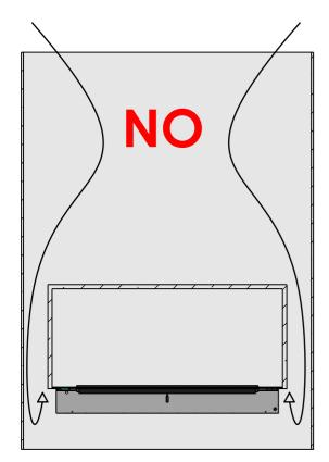
DO NOT! install the fireplace in a wall construction which is open above and below the fireplace. The warm air will cause turbulences inside this hollow construction which will have a negative impact on the flames.
