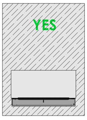
DO! install the fireplace in a massive wall (made of bricks, stone or gas beton) using the wall cut-out dimensions mentioned on the previous page.
