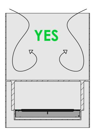
DO! install the fireplace in an open-wall construction, which is closed above and below the fireplace. Make sure to create a closed cavity for the section below the base plate of the fire.
