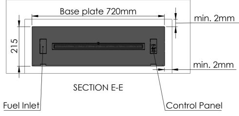
Please Note, if using the minimum required dimensions for the wall cut-out, the wall in front of the safety chamber becomes very thin, only 7,5mm.
